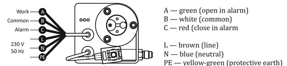
Fig.3. Electrical Connection
